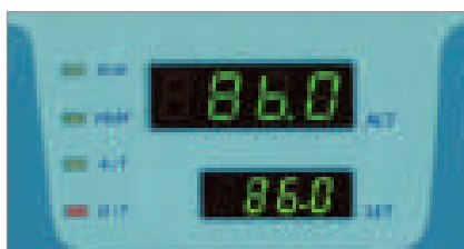
Simultaneously displays set temperature and actual temperature.
