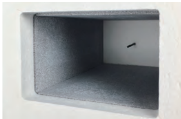
1100°C model (4-side molding type heater)
