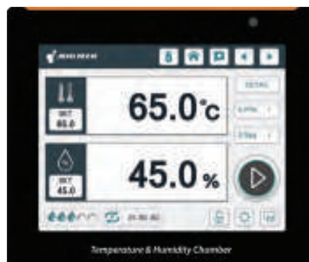
Color touch display controller (5.6 inches)
