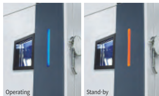
Indicator LED of operation condition
