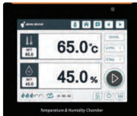
Large LCD touch screen controller (5.6 inches)
