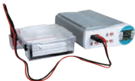
Connection to Power Supply
