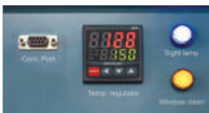
Electronic over temperature shutdown system.
