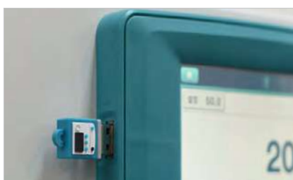
Data storage using USB ports
